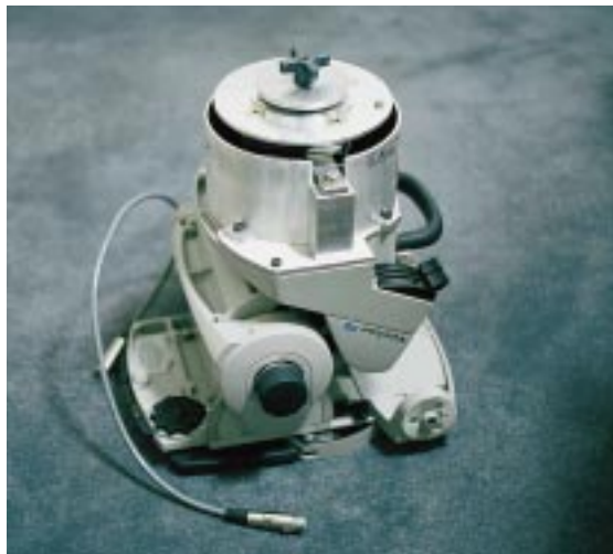
2 An instrumented tripod head for the broadcast camera, sitting upside down to show the encoders added to read out pan and tilt.
