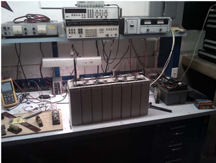
Eight CALB CA180FI cells, during initial balancing with all cells in parallel. 50A, current limited, remote sensing, lab power supply is in the upper right.
