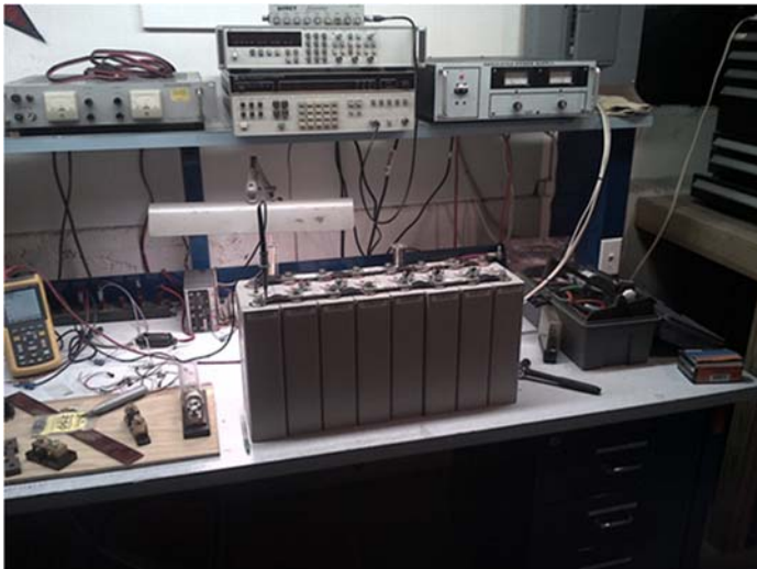
Eight CALB CA180FI cells, during initial balancing with all cells in parallel. 50A, current limited, remote sensing, lab power supply is on the right side of the upper shelf.
